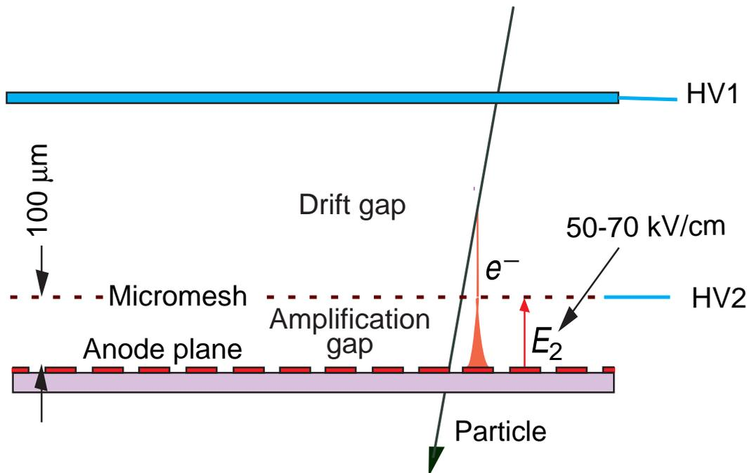
Figure 35.11: Schematic drawing of the Micromegas detector.
