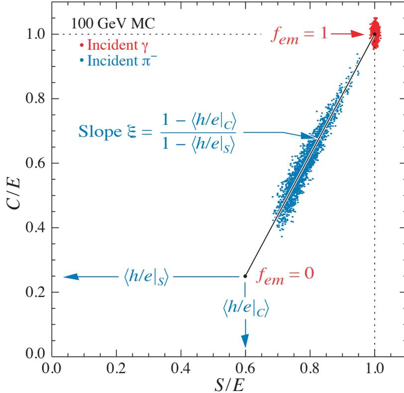
Figure 35.23: Scatter plot of Monte Carlo  $C/E$  (Cherenkov) vs  $S/E$  (scintillator) signals for individual events in a dual readout calorimeter. Hadronic events are shown in blue, and scatter about the indicated event locus. Electromagnetic events cluster about  $(C/E, S/E) = (1,1)$ . In this case worse resolution (fewer p.e.'s) was assumed for the Cherenkov events, leading to the “elliptical” distribution.
