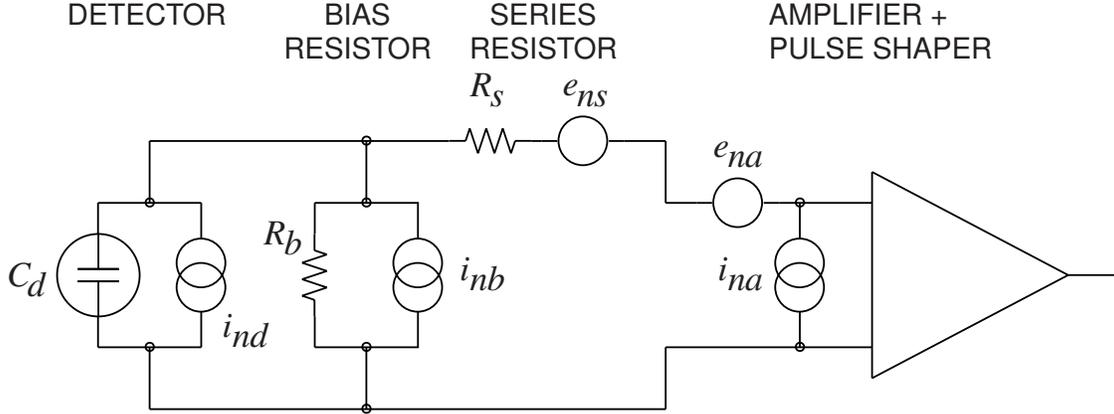
Figure 35.19: Equivalent circuit for noise analysis.
