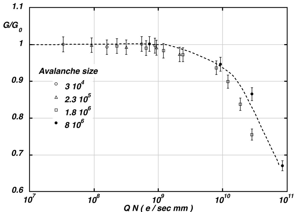
Figure 35.8: Charge rate dependence of normalized gas gain  $G/G_0$  (relative to zero counting rate) in proportional thin-wire detectors [111].  $Q$  is the total charge in single avalanche;  $N$  is the particle rate per wire length.
