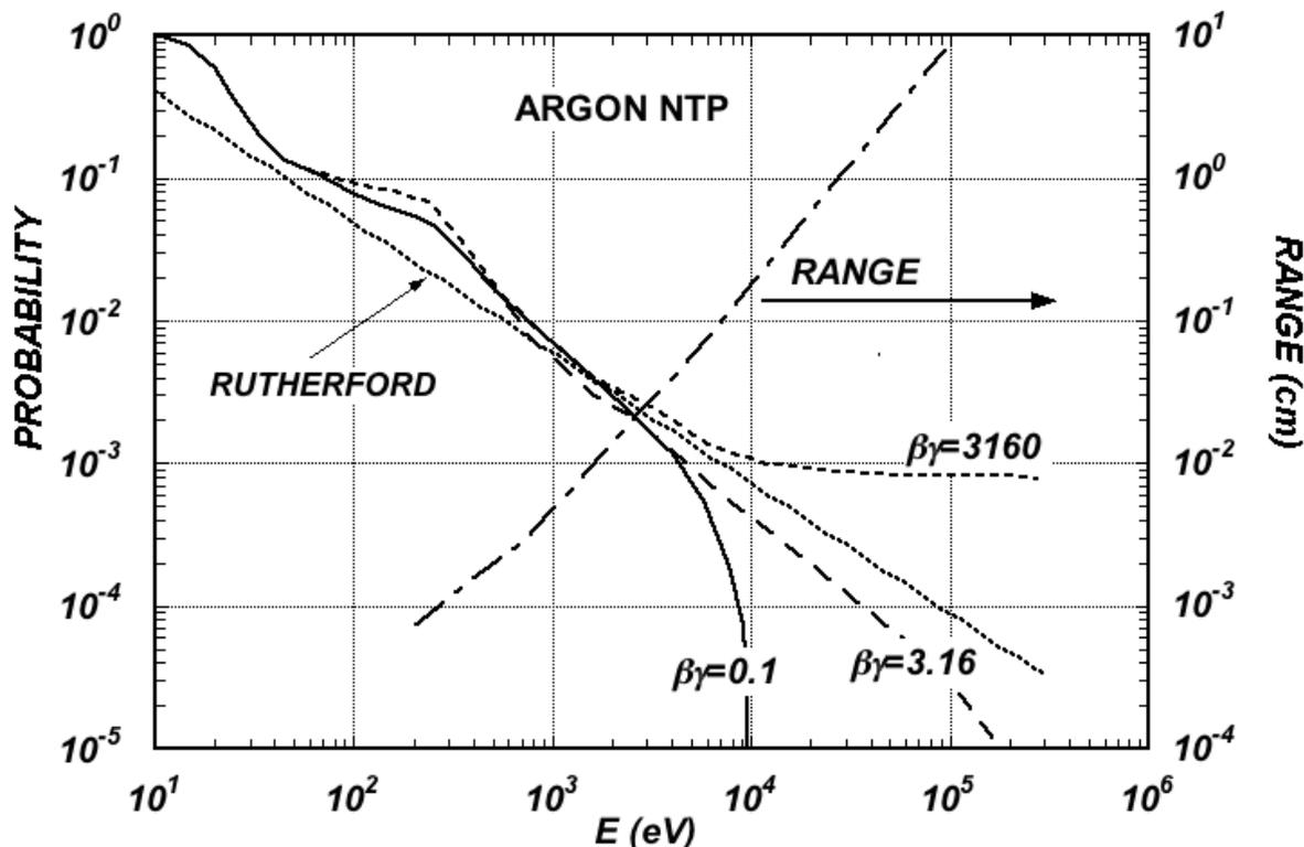
Figure 35.3: Probability of single collisions in which released electrons have an energy  $E$  or larger (left scale) and practical range of electrons in Ar/CH<sub>4</sub> (P10) at NTP (dot-dashed curve, right scale) [88].
