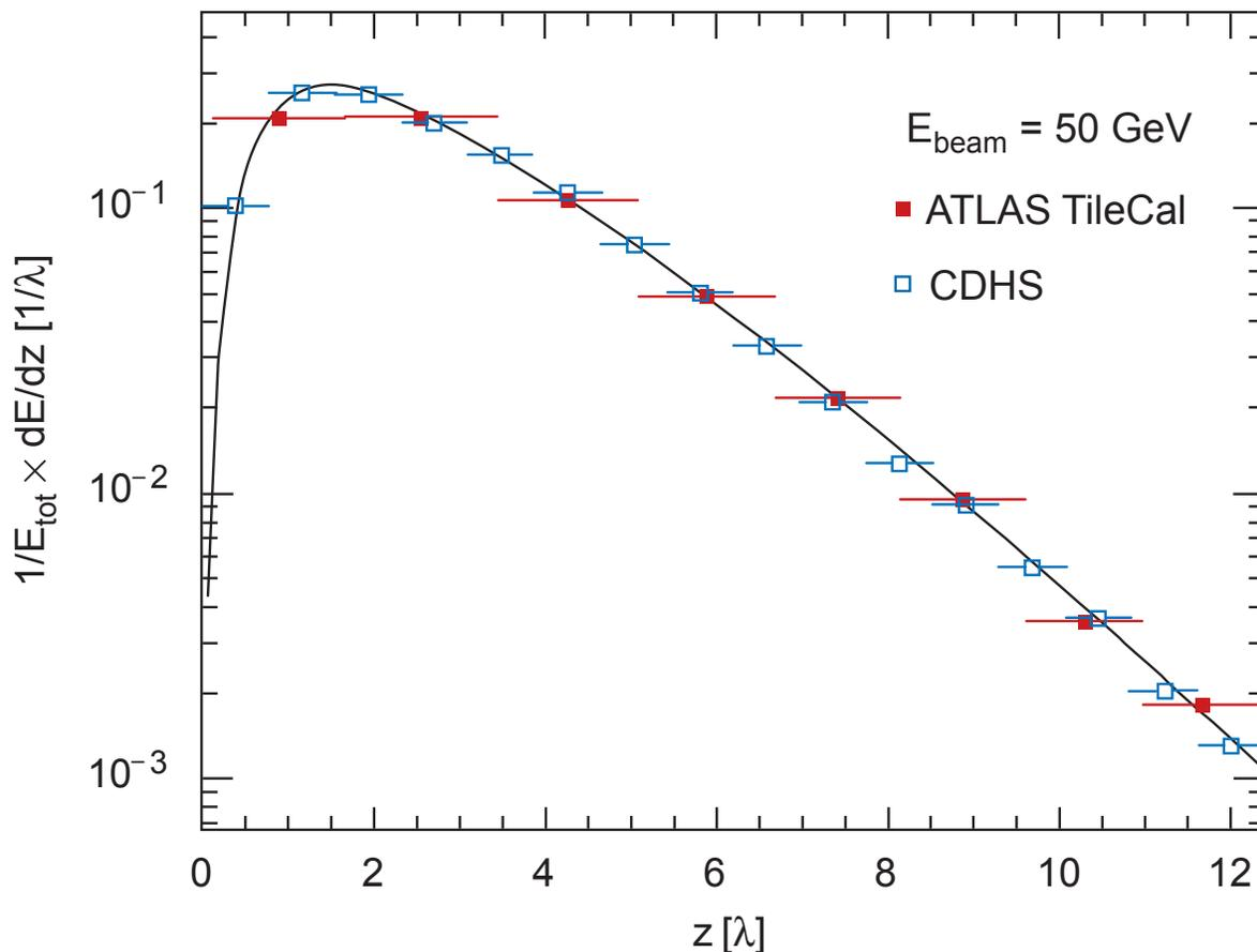
Figure 35.24: Mean profiles of  $\pi^+$  (mostly) induced cascades in the CDHS neutrino detector [255] and in the ATLAS tile calorimeter [224]. Measurements are front of the calorimeter, and so are convoluted with the first interaction distance.
